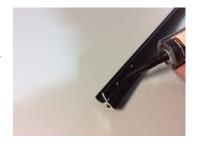
Step Six Apply a tiny amount of the sealant over each pre-drilled hole in the van. With the help of an assistant, hold the rail in position being very careful not to smudge the sealant bead. Fix the rail into the pre-drilled holes with your PH2 hand screwdriver using the supplied black stainless steel screws. Again, start from the middle, work towards the front, and then from the middle towards the rear. TAKE CARE NOT TO OVER TIGHTEN THE SCREWS the sealant is the main fixing once cured.
