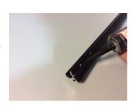
Step Six Apply a tiny amount of the sealant over each pre-drilled hole in the van. With the help of an assistant, hold the rail in position being very careful not to smudge the sealant bead. Fix the rail into the pre-drilled holes with your PH2 hand screwdriver using the supplied black stainless steel screws. Again, start from the middle, work towards the front, and then from the middle towards the rear. TAKE CARE NOT TO OVER TIGHTEN THE SCREWS the sealant is the main fixing once cured.
