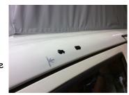
**Step Seven** Dry fit the front rubber profile following the contours of the van, put a pencil reference mark when happy with position. Peel the red backing from the 3M tape and carefully fix into place following the reference mark - YOU ONLY GET ONE CHANCE! Press firmly into place all the way along. Mask around and seal with Sikaflex.
